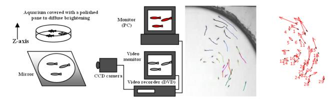
Figure 1. Left: Diagram of the multitracking setup. A CCD camera filmed a mirror reflecting the bottom of the circular tank. Right: example of tracks (detail of the arena, period of 1 sec) and the same image with individual assignments and velocity speed.
