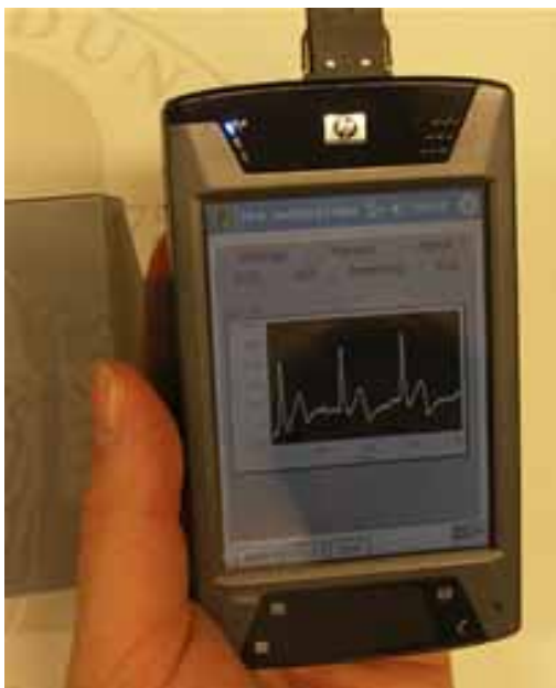
Figure 1. Left side: Photo of the PDA based Physiology monitor; Right side: Examples of high quality data acquired with the PDA based Physiology monitor
