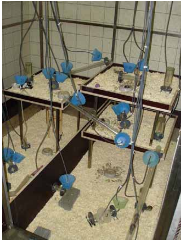
Figure 1. Semi-naturalistic environment (SNE). RFID marked mice were automatically tracked when passing a ring-antenna.
