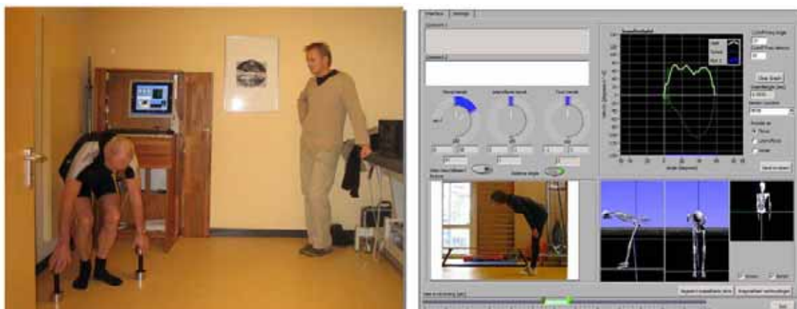
Figure 2. Left: Real time viewer beta-GUI example for an application aiming at improving training of specific low back pain patients towards more favorable back use (IC-Coach) Clinical relevant info (ROM, kinematics phase plot) are shown synchronized with context data (video + 3D avatar). Right: Using this real-time application a patient is coached in balancing load exposure of her lower back by a physical therapist in a back school program
