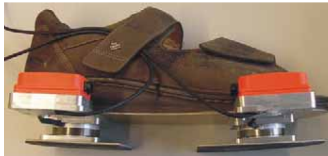
Figure 1. Picture of the forceshoe with two force/moment sensors beneath the heel and the forefoot and two inertial sensors rigidly attached to the force/moment sensors.
