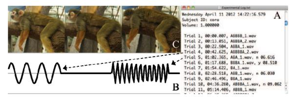
Figure 2. Sketch of the sonification procedure. Using a Python script, each event in the experimental log (A) is transformed into one or more sounds chosen by the researcher. The resulting soundtrack (B) is joined with the original video (C) and these are played simultaneously during behavioral coding. (Squirrel monkey pictures by Markus Boeckle)
