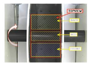
Figure 3. Top view image of one lane of the rotarod. Overlays show the area of interest (red) and the 3 distinct individual zones (yellow) covering the rod (mid) and the front and back zones as determined in EthoVison® XT. The width of the red area was set to the width of one lane of the rotarod and the length was set to 3.7 times the diameter of the rod. The arrow indicates turning direction of the rod.
