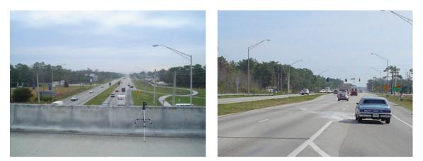
Figure 3. Video camera positioned on the bridge and road tubes placed every 100 feet along the arterial.
