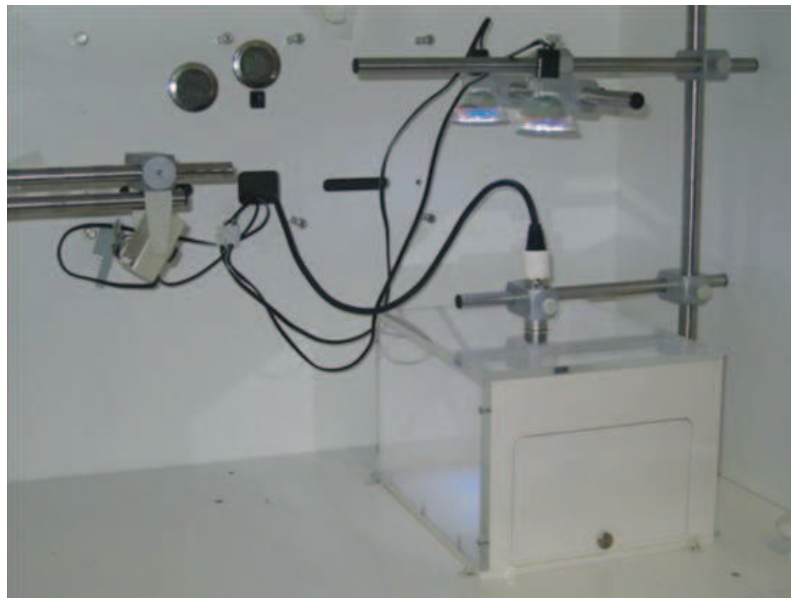
Figure 1. Setup for measuring isolation-induced ultrasonic vocalizations in rodent pups. The roof and one wall are made of transparent plastic to allow video observation during the test. The isolation box is placed in a sound attenuating isolation cubicle (51x71x51 cm; Coulbourn Instruments, Allentown, USA) equipped with 2 white-light LED spots (63 lux, Conrad Electronic GmbH, Hirschau, Germany) and a black/white CCD camera (Conrad Electronic GmbH) connected to a DVD recorder (DVR-3100 S, Pioneer, Willich, Germany).
