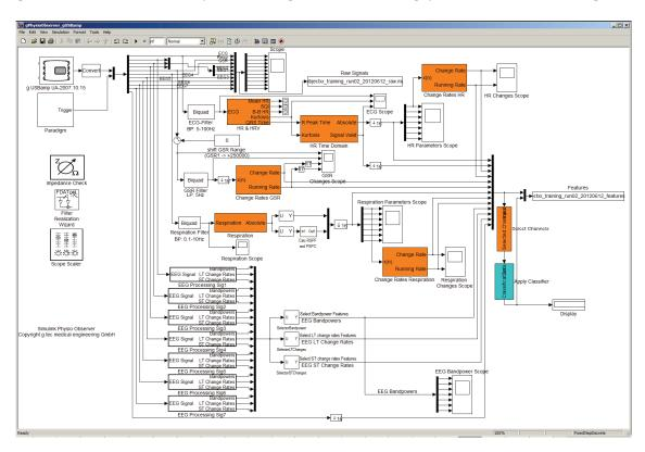
Figure 1. The g.PhysioObserver system allows to assess and evaluate different mental and physical sates of a subject online in real-time based on physiological signals and features extracted thereof.
