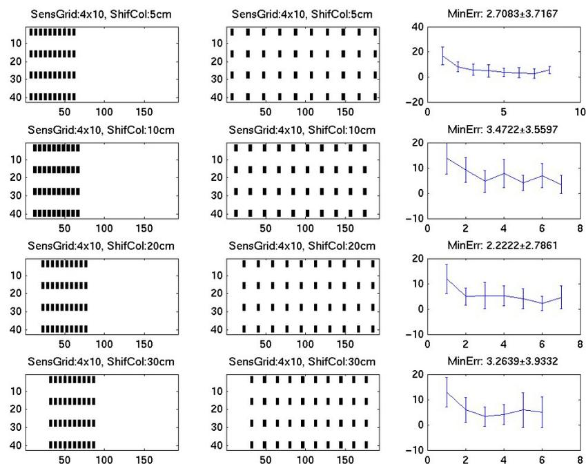
Figure 4. Sensor grid optimization by changing the distance between sensors.
