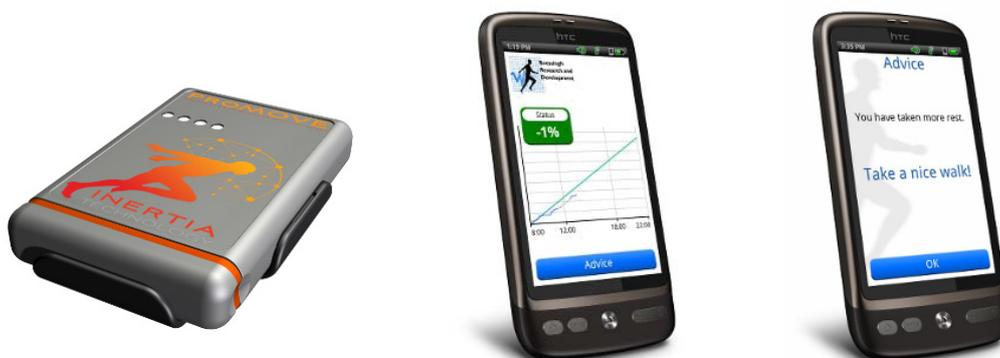
Figure 1. The Activity Monitoring and Feedback system from Roessingh Research and Development. Depicted is the ProMove-3D activity sensor, and two screenshots of the Smartphone interface showing a graph of daily activity and a motivational message.
