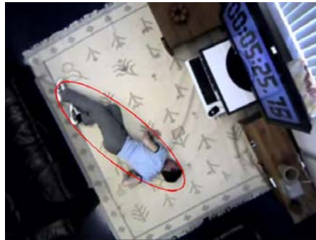
Figure 1. Skeleton as derived from Kinect depth image. Figure 2. Bounding ellips extracted from foreground segmentation
