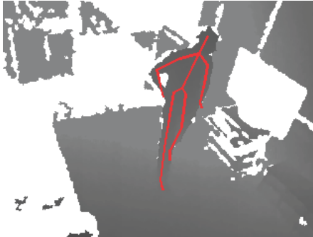
Figure 1. Skeleton as derived from Kinect depth image. Figure 2. Bounding ellips extracted from foreground segmentation
