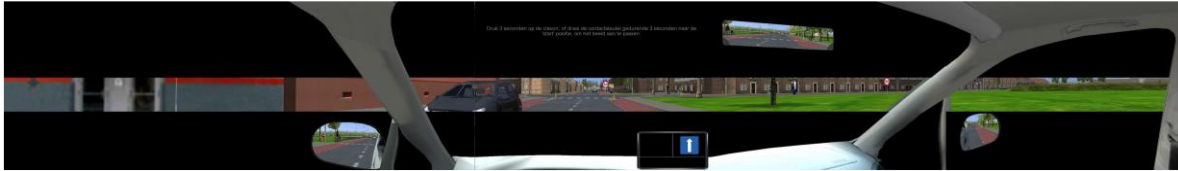
Figure 3: the vertical FOV is minimized with wide screens monitors and black areas
