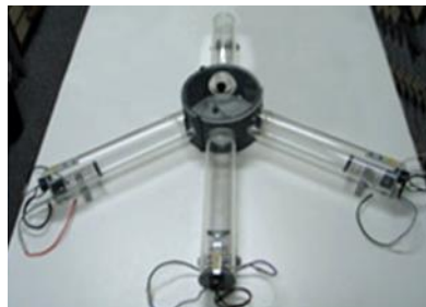
Figure 1: The TPL maze. Mice are food deprived to 85% of ad libitum feeding weight, but can find food at the end of each of the maze arms, behind a small metal grid. In each of the 3 daily sessions (lasting maximally 10 min per mouse), mice have to learn to avoid 1 of the 3 feeding locations, depending on the time of day (i.e., session). On visiting a 'wrong' location, mice receive a mild but aversive foot shock (<1 s).
