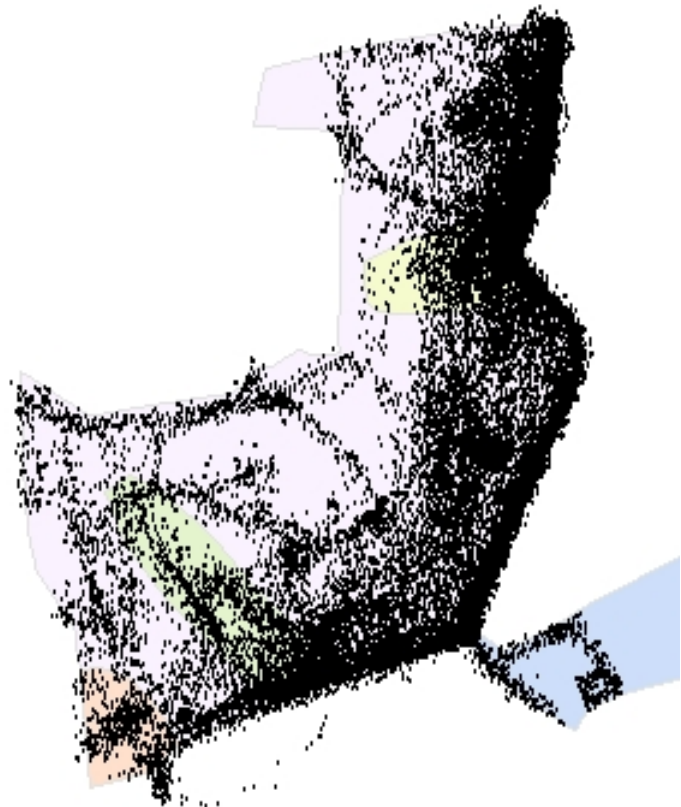
Figure 2. Pattern of paddock utilization by a group of 12 cows over one month in January 2013 based on i-gotU (Mobile Action, Taiwan) GPS device operating with 10 s sampling interval.
