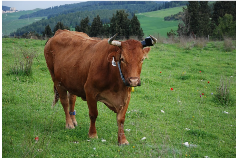
Picture 1. Cow wearing pedometer (rear, left leg), GPS collar and acoustic sensor (black box on left horn) in a paddock of herbaceous rangeland vegetation at Kibbutz Ein Hashofet, Israel.
